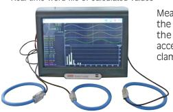
Measurements are done with the voltage input (direct) of the unviversal board and accessories clamps (standard clamps or flexible clamps)
