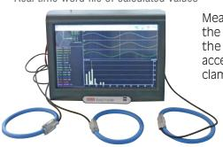
Measurements are done with the voltage input (direct) of the unviversal board and accessories clamps (standard clamps or flexible clamps)
